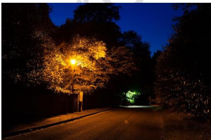
Figure 6 – old style sodium street light scatters light in all directions whilst new style LED (in distance) directs all light down below the horizontal. Note pool of light on ground.
